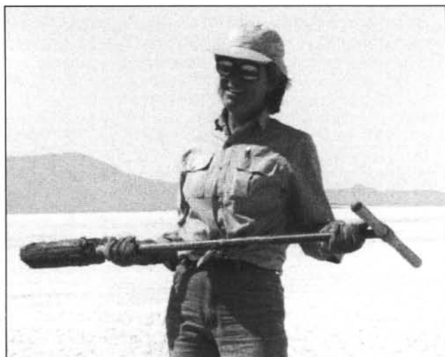
Figure 7. Hand auger for collecting water and sediment samples on playa, east of Summer Lake. (See also cover photo.) Location is auger site L; view is to the northwest.
