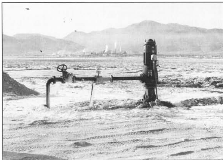
Figure 8. Brine well on Searles Lake, California. View toward northwest shows Trona plant of North American Chemical in the distance.
