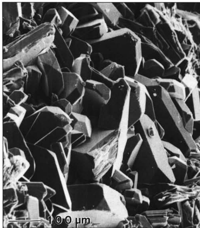
Figure 3. Scanning electron micrograph of randomly oriented, tabular to blocky, euhedral heulandite crystals from about 771 m.
