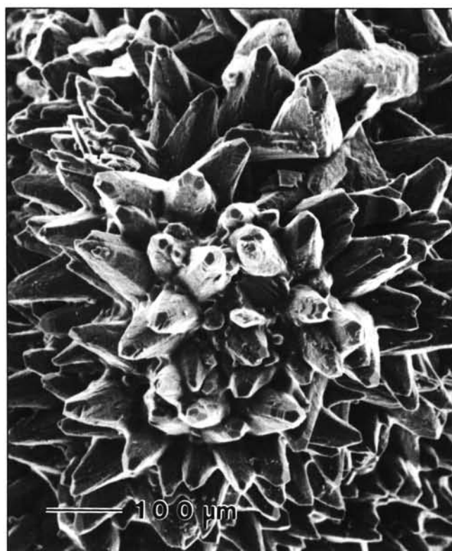
Figure 10. Scanning electron micrograph of drusy subhedral quartz crystals that formed in a fracture or cavity filling at about 802 m.
