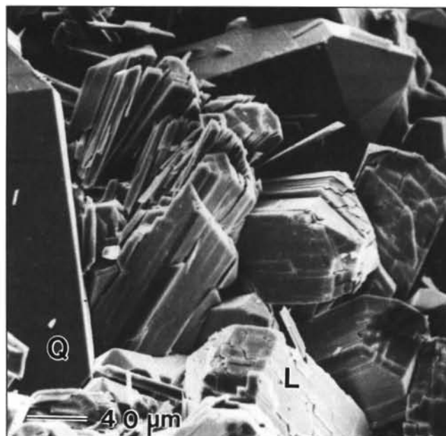
Figure 4. Scanning electron micrograph of fractured to broken laumontite (L) crystals in association with earlier, euhedral quartz (Q) crystals from about 1,454 m. See also Figure 8.
