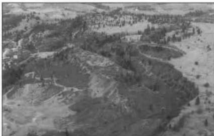
Figure 1. Mosier Quarry properties, aerial view to the east. Aggregate mining on ODOT property developed headscarp right of center. Photo courtesy of Landslide Technology, Division of Cornforth Consultants, Inc., Portland.
