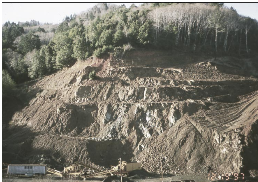
Freeman Rock operation, showing stable, benched highwall. The operator was recognized for outstanding stormwater control and slope stabilization.
