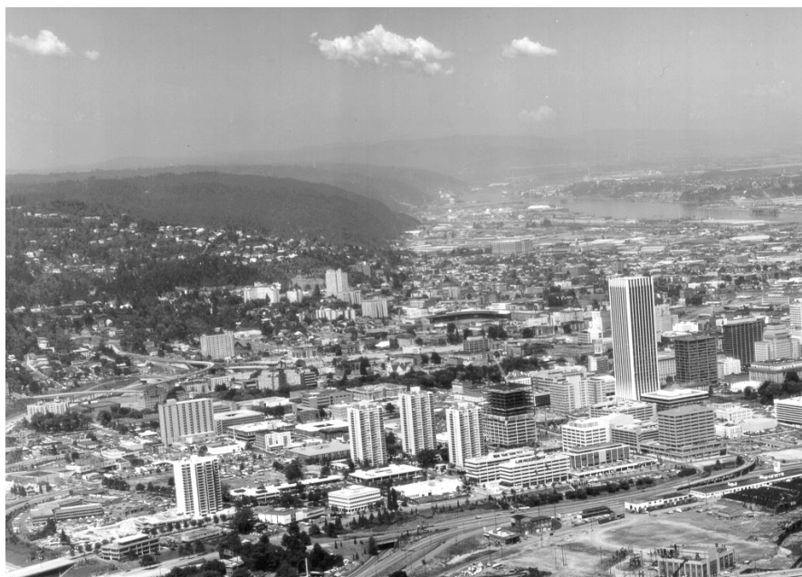
Two major north northwest-trending faults slice across Portland. The Portland Hills fault to the left is marked by the straight northeast margin of the foothills, while across the Willamette River, the parallel East Valley fault is buried beneath alluvium and fill. Photo courtesy of Delano Photographics.
