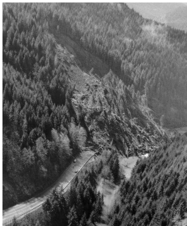
On the Wilson River in Tillamook County, a 1991 landslide completely covered Highway 6 and dammed the stream. Clean-up took two months. Photo courtesy of Oregon Dept. of Transportation.
