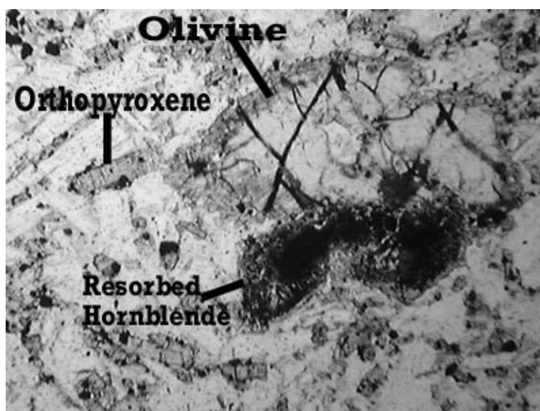
Figure 4. Thin section photomicrograph of hornblende-olivine textural relationship in a 5.6-m.y.-old andesite flow. Image is 3mm x 2mm.
