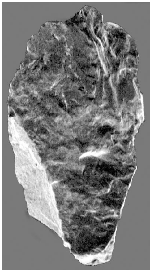
Figure 3. Scanning electron photomicrograph of a plutonic detrital quartz grain derived from Mount Ashland granodiorite. Grain is approximately 1.0 mm in length.
