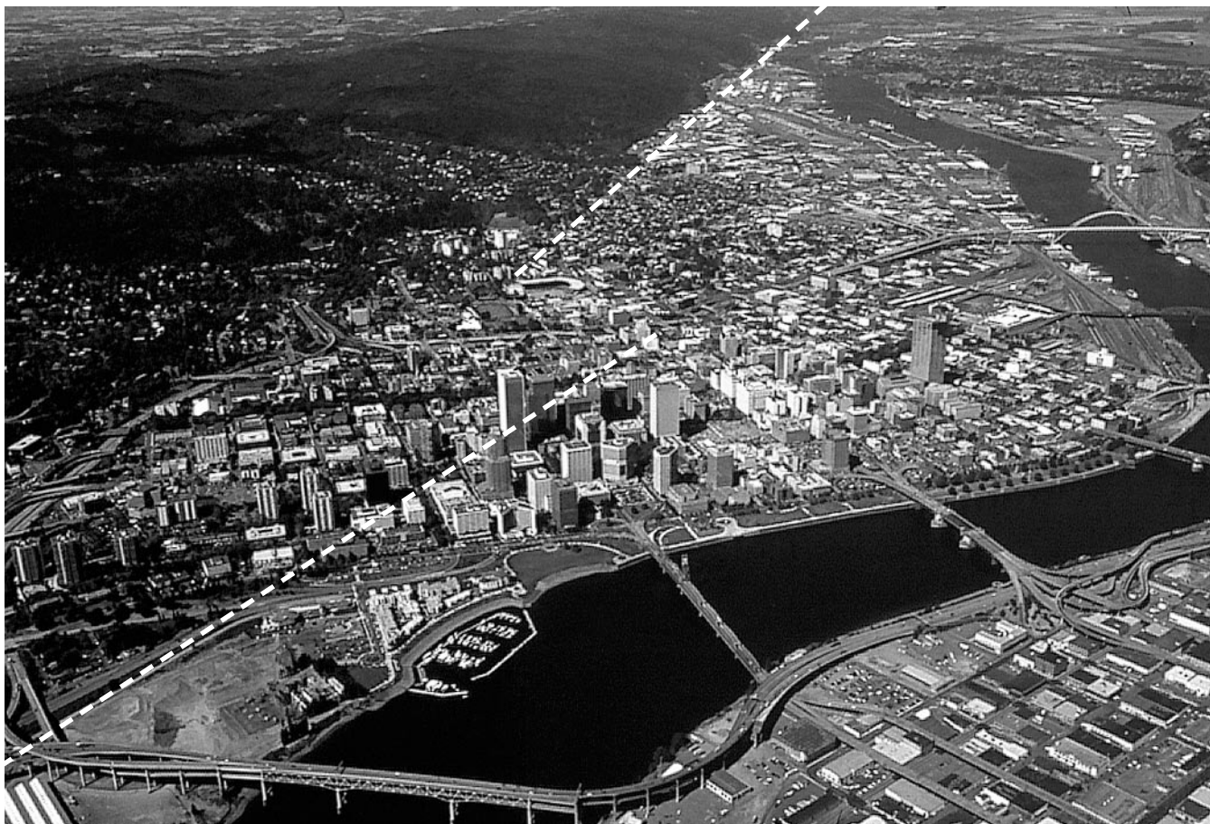
Figure 1. Oblique air photo of the Portland Hills toward the northwest and inferred location of the Portland Hills fault. The fault is mapped near the eastern base of the escarpment north of West Burnside Street. To the south, the inferred fault steps toward the east, where it traverses the downtown area and crosses the Willamette River (Figure 2). Fault location based on Madin (1990). Air photo courtesy of Northern Light Studio.
