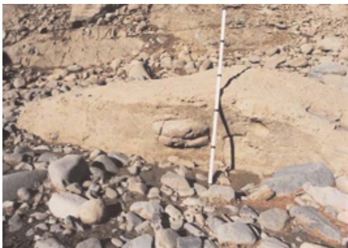
Figure 7. Unit A, poorly sorted, matrix-supported basal till. 1.5 meter staff for scale.
