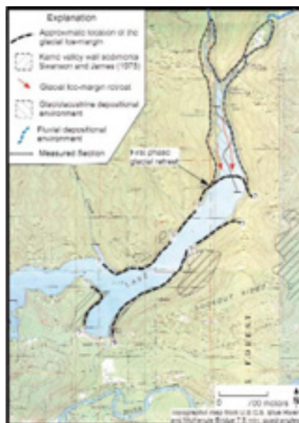
Figure 21. First Phase glacial retreat. Deposition of glaciolacustrine sediments (Unit B) in a closed system.
