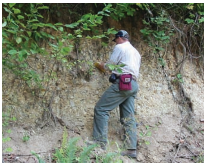
DOGAMI Baker City Field Office geologist Jason McClaughry takes a statistical point count of the composition of the cobbles in a conglomerate unit near Lebanon, Oregon, as part of the Middle Willamette geologic mapping project for the U.S. Geological Survey STATEMAP program. Field observations provide information about the source area and possible relative age of the unit.
