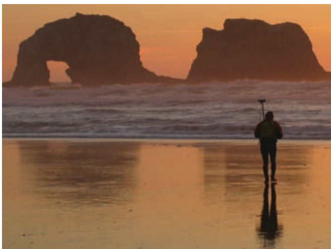
DOGAMI Coastal Office-U.S. Army Corps of Engineers partner Lindsey Gay takes measurements at Rockaway Beach. Regular monitoring at a network of sites along the Oregon coast helps us understand the effects (erosion or accretion) of storms and improves our understanding of long-term coastal change due to sea level rise and climate change.
