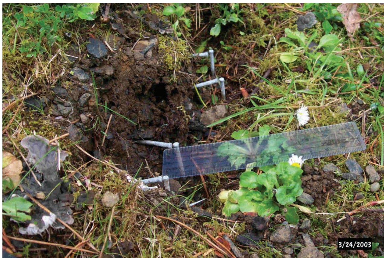
Figure G1. A typical marker nail site (JC-23 ); 6-in ruler used for measurements.
