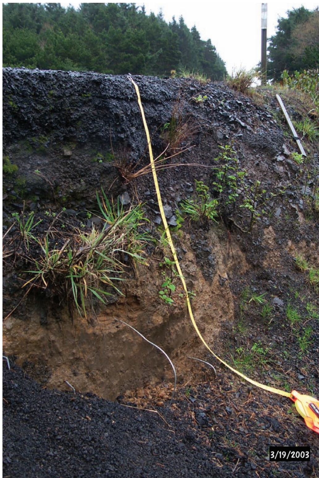
Figure G15. Marker nail site JC-23 with both wires and nails, looking south southeast. Scarp is in red orange fill of excavated Astoria Formation overlain by gravel and asphalt. Near vertical portion of scarp is ~1.2 m high.
