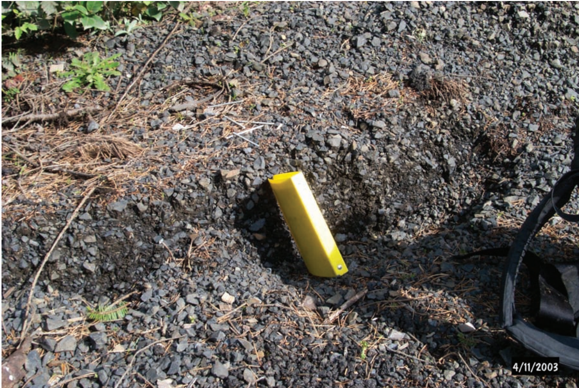
Figure G12. Marker nail site JC-21 looking southeast. Yellow field book is ~19 cm long. The scarp is in gravel fill from the Highway 101.
