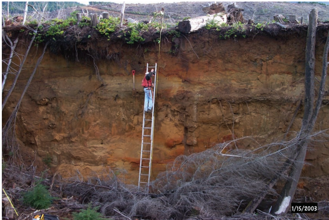
Figure 13. Pleistocene marine terrace sand exposed in the northeast headwall of the landslide. Jonathan Allan of DOGAMI is measuring the thickness of the unit. Note the nearly flat surface of the sand sheet. The contact with underlying Tertiary Astoria Formation is ~1 m below the base of the ladder.
