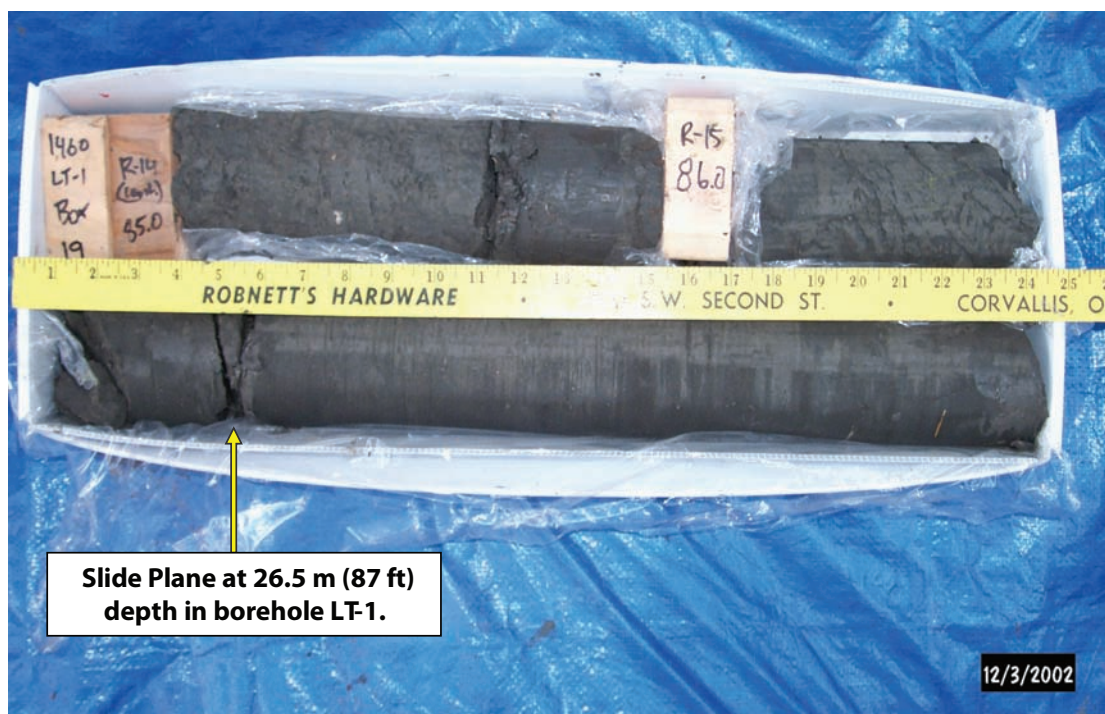
Figure 18. Core at the slide plane from the western (LT-1) inclinometer hole. Numerous sheared fractures occur just above the slide plane.
