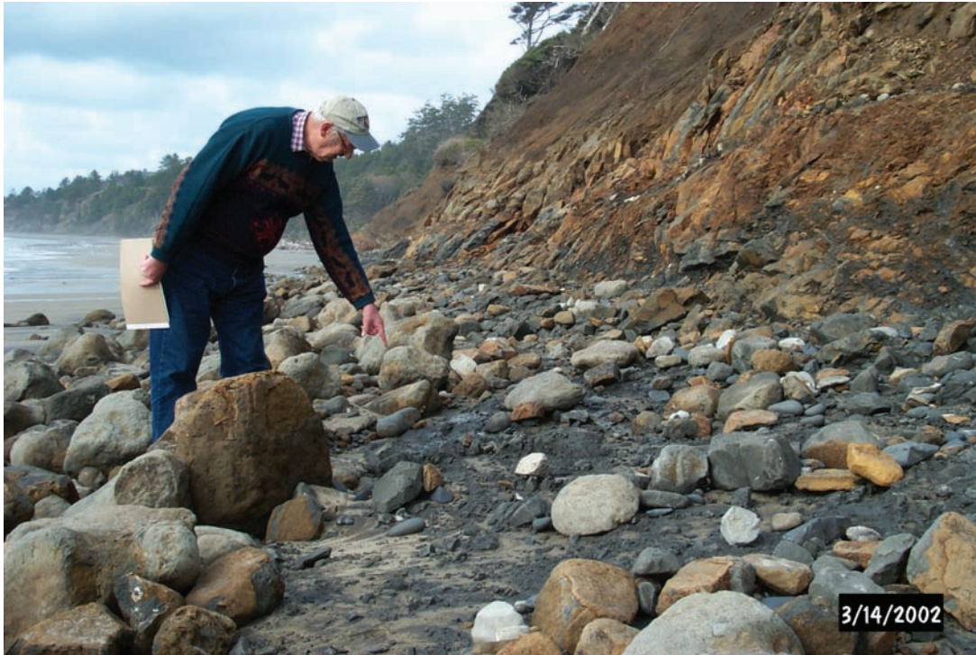
Figure 12. Highly sheared dark gray sandy siltstone unit at the toe of the Johnson Creek landslide. This unit underlies the tan sandstone in Figure 3. Chuck Dennison of Dennison Surveying is pointing at the unit. Slightly reworked talus from the slide partially covers the basal shear zone.
