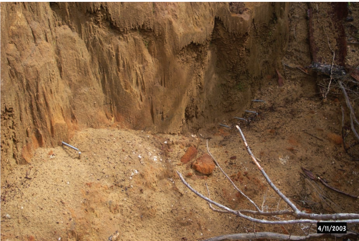
Figure G17. Marker nail site JC-24 looking southeast. This is the northeast headwall of the landslide. The tan unit in the near vertical escarpment is Pleistocene marine terrace sand. Talus lies along the base of the slope.
